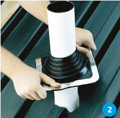
2 Slide Master Flash® down the pipe (a non-petroleum base lubricant will ease installation).
