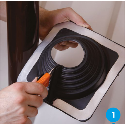
1 Select an appropriate Master Flash® Multi. If necessary trim opening to the pipe diameter.
